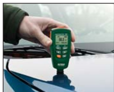
Measuring the thickness of automotive paint
