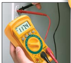
Displays AC Voltage of an outlet receptacle
