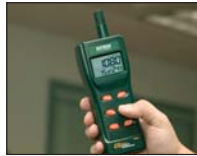
Measure CO 2 level in office buildings to insure proper ventilation.
